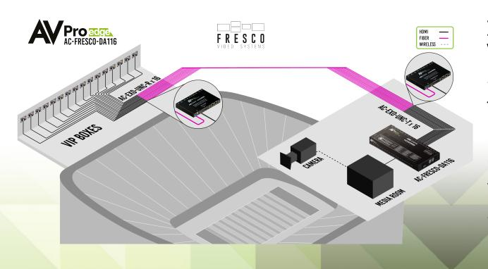
The Fresco 1x16 delivers a completely uncompressed video signal. That means you can deliver true 4K HDR or Dolby Vision video along side full bitstream audio like Dolby Atmos or DTS HD throughout the HDMI input and outputs. Many video distribution solutions use compression to make delivering the video signal easier, but this can degrade and pixelize the image. Choosing the Fresco repeater allows you to deliver the most optimized picture available to each display in the installation.
