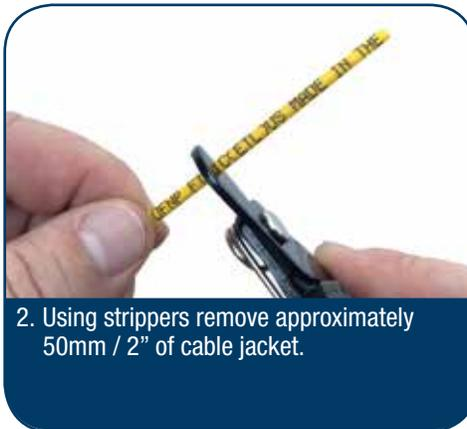
2. Using strippers remove approximately 50mm / 2" of cable jacket.
