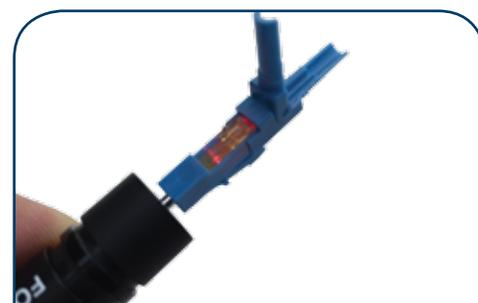
3. Place onto VFL using an LC type adapter. Ensure activator slide tab is in "open" position - slide towards rear of connector. Open hinge on connector.
