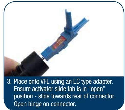
3. Place onto VFL using an LC type adapter. Ensure activator slide tab is in "open" position - slide towards rear of connector. Open hinge on connector.
