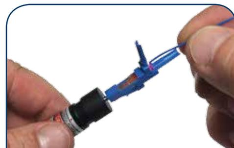
6. Insert fiber into the rear of connector until a slight "bow" is created and the light emitting from connector window dims and/or extinguishes.
