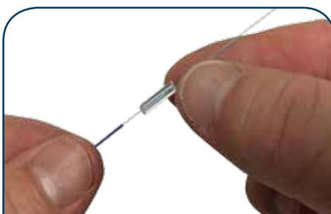
2. Slide included 900µm build tube section onto fan tubing.
