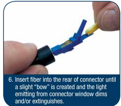
6. Insert fiber into the rear of connector until a slight "bow" is created and the light emitting from connector window dims and/or extinguishes.
