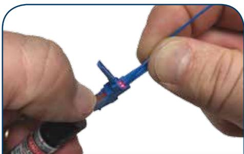
7. Slide activator tab towards connector tip. Remove from VFL, Install dust cap.
