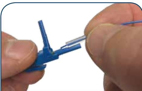
8. Slide build tube forward and seat in rear of connector, ensure fiber is straight, close hinge. Slide boot forward and tighten until secure.
