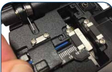
5. Cleave fiber measuring from fan tubing. For SSF™ LC = 12mm.<sup>2</sup>
