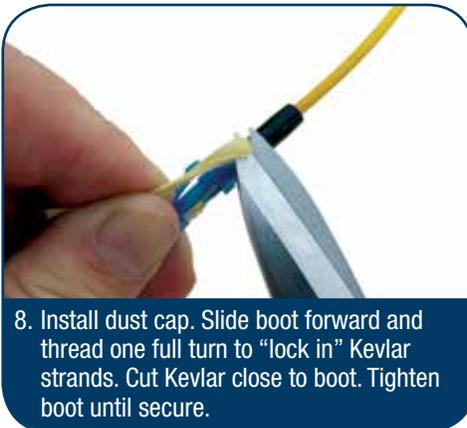
8. Install dust cap. Slide boot forward and thread one full turn to "lock in" Kevlar strands. Cut Kevlar close to boot. Tighten boot until secure.
