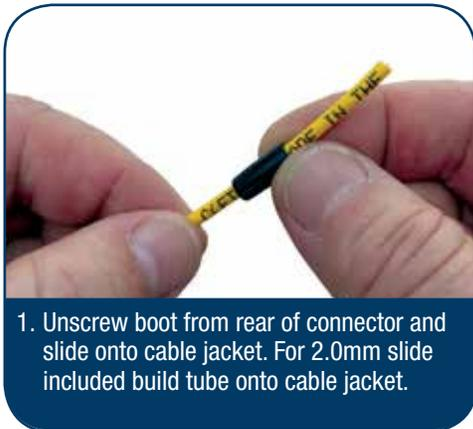
1. Unscrew boot from rear of connector and slide onto cable jacket. For 2.0mm slide included build tube onto cable jacket.
