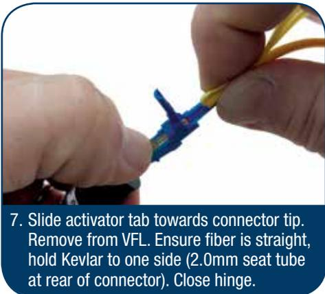
7. Slide activator tab towards connector tip. Remove from VFL. Ensure fiber is straight, hold Kevlar to one side (2.0mm seat tube at rear of connector). Close hinge.
