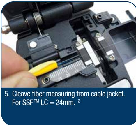
5. Cleave fiber measuring from cable jacket. For SSF™ LC = 24mm. <sup>2</sup>
