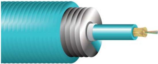
Cleerline SSF™ micro distribution Aluminum Interlocking Armored cable consists of either a Riser or Plenum overall jacket with 2-72 fibers and water blocking Kevlar® yarns. All Aluminum Interlocking Armored is indoor rated.
