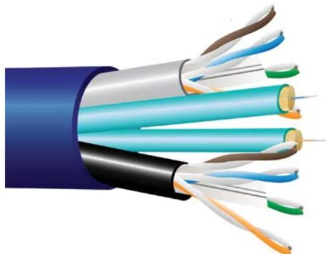
Cleerline SSF™ Fiber & Category cable is composed of two simplex OM3 fibers with two Category 6 cables.
