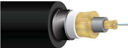
Cleerline SSF™ Armored Corrugated Steel Distribution cable consists of a PE overall jacket with 2, 6, or 12 fibers and water blocking Kevlar yarns.
