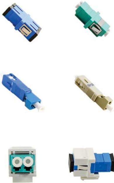
SSF™ Fiber Optic Feedthrough Adapters provide easy cable connections. Available in simplex and duplex SC/SC and LC/LC configurations for single mode (OS2 or 9/125 μm) and multimode fibers (OM2, OM3, OM4 or 50/125 μm).
