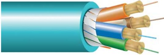
Cleerline SSF™ 2-4 strand fiber Breakout type cable is composed of SSF™ fibers in an overall jacket with 2.0 mm subunits and if applicable, a central strength member.
