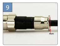
The cable mark from step 5 should line up with the back edge of the compression ring.
