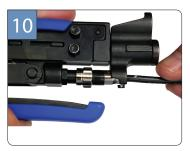
Using your VT-200 compression tool, make sure the rotating compression head is positioned for 6/59 as shown in the picture. Properly seat connector and compress fully.
