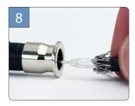
Insert the cable into the back of the connector with the step up pin and insulator guide inside the post. Push the connector on while rotating until fully seated.
