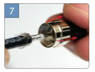
Once the center conductor is pressed fully into the pin pull the connector away from the cable. The step up pin and insulator guide will stay with the cable as shown.
