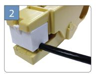
Using a fixed blade, mini prep tool in good condition, prepare cable to 1/4" x 1/4" dimensions. Use edge of tool if no stop
