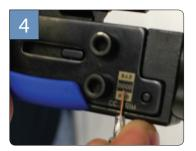
Ensure cable preparation is correct. Use gauge on VT tool to check the center conductor length.
