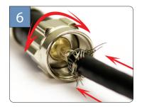
Insert cable center conductor into the pin stored within the nut of the connector. Push into the pin while rotating the connector.
