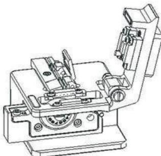
**Preparing fiber involves removal of colored soft peel coating per instruction steps included with SSF™ connectors. Do not attempt to cleave fiber that has not been prepared.**
