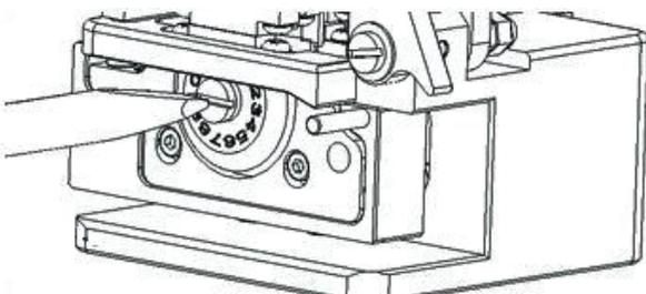
1. Unscrew the screw that connects the blade carriage sliding block.
