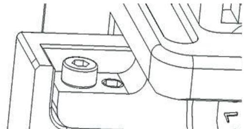
2. Loosen the blade clamping screw.
