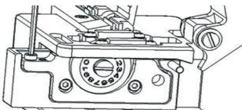
If fiber does not cleave, ensure all steps have been followed prior to adjustment. Refer to SSF™ adjustment procedure included with this cleaver.
