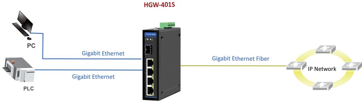
**HGW-401S Gigabit Ethernet Switch Application**
