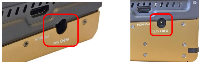
Figure 14: MS103TDs and MS104B Input Powering Sockets
