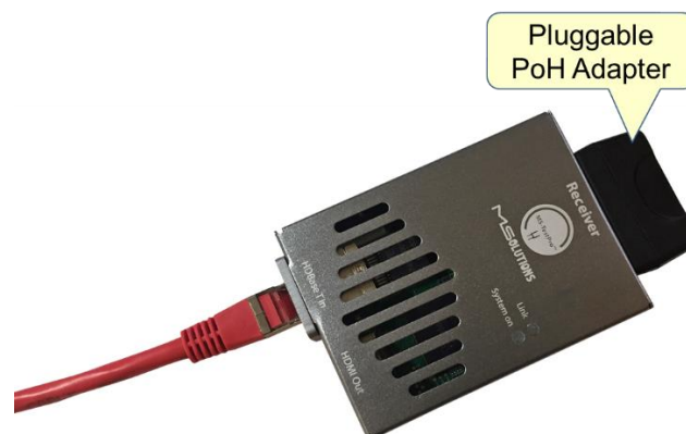
Figure 13: Pluggable PoH Adapter on Remote Module
