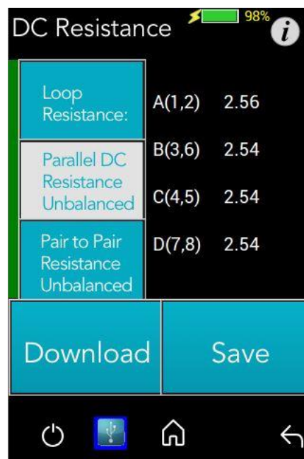
Figure 51: Parallel DC Resistance Unbalanced Results
