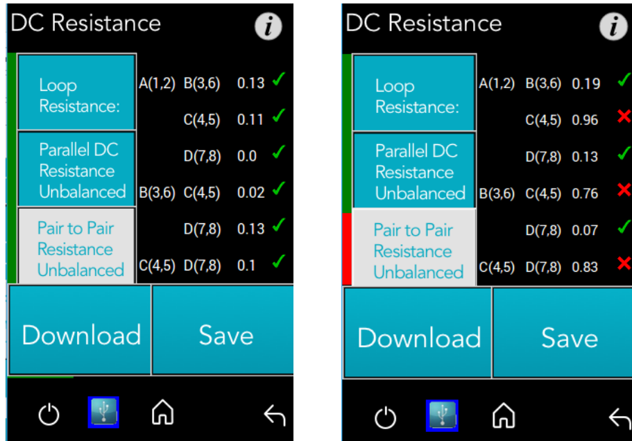
Figure 52: Pair-to-Pair Resistance Unbalanced Results
