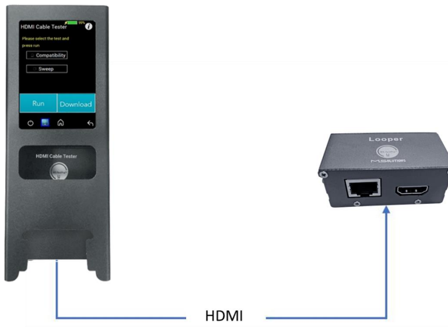
Figure 119: HDMI Cable Tester Setup
