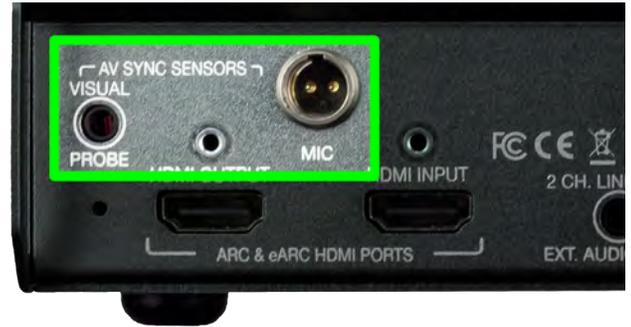
**Microphone** - This mini-XLR connection is where you connect the included microphone for audio or audio/video latency tests. After connecting the microphone to the SEVEN-G-8K, place the microphone as close to the display's speaker (or a speaker in the audio system) as possible.
