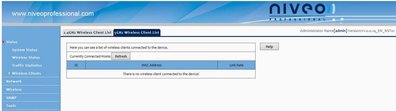
1. **MAC Address:** Displays connected wireless client's MAC address.
