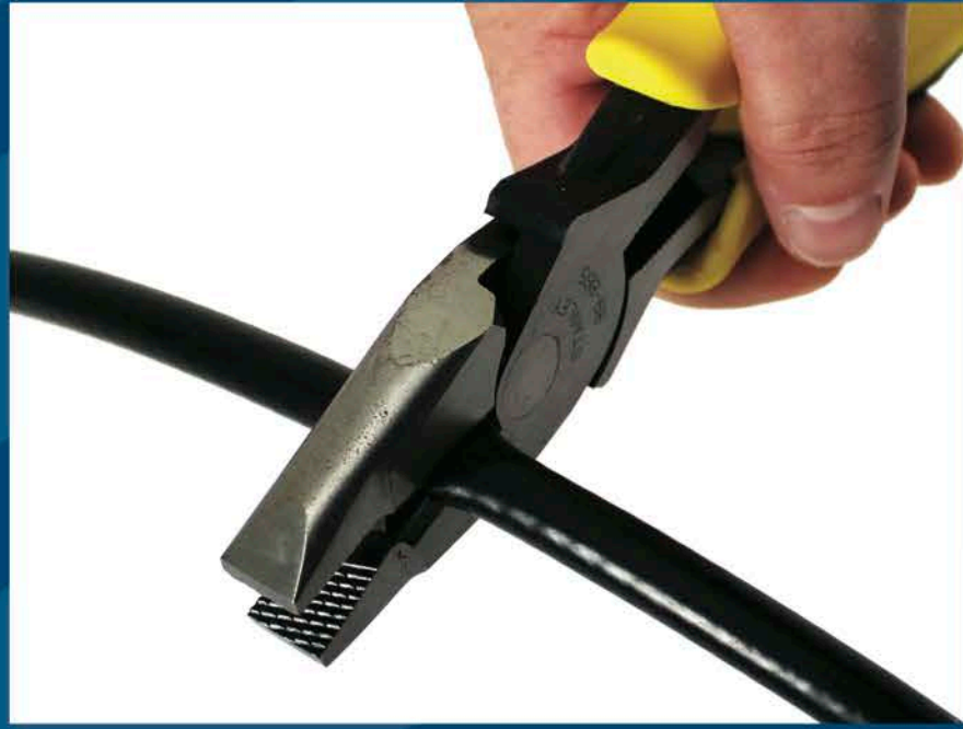
Cut cable squarely
