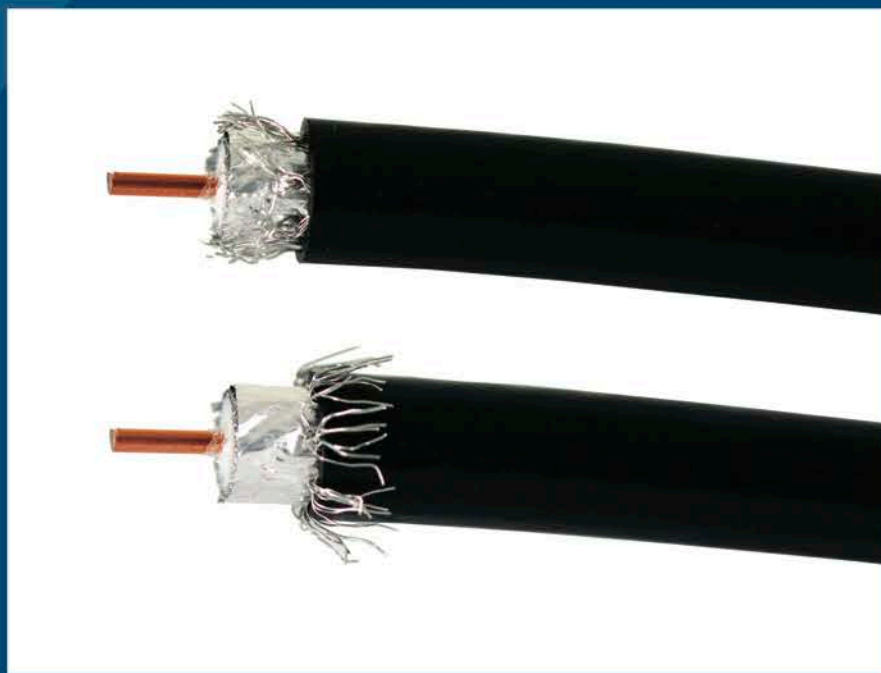
Ensure there is no dielectric, braid or foil wrapped around center conductor. Fold back braid.
