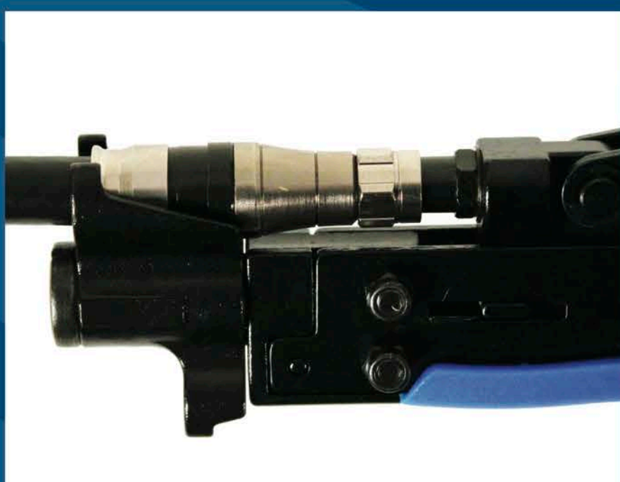
Properly seated connector ready for compression
