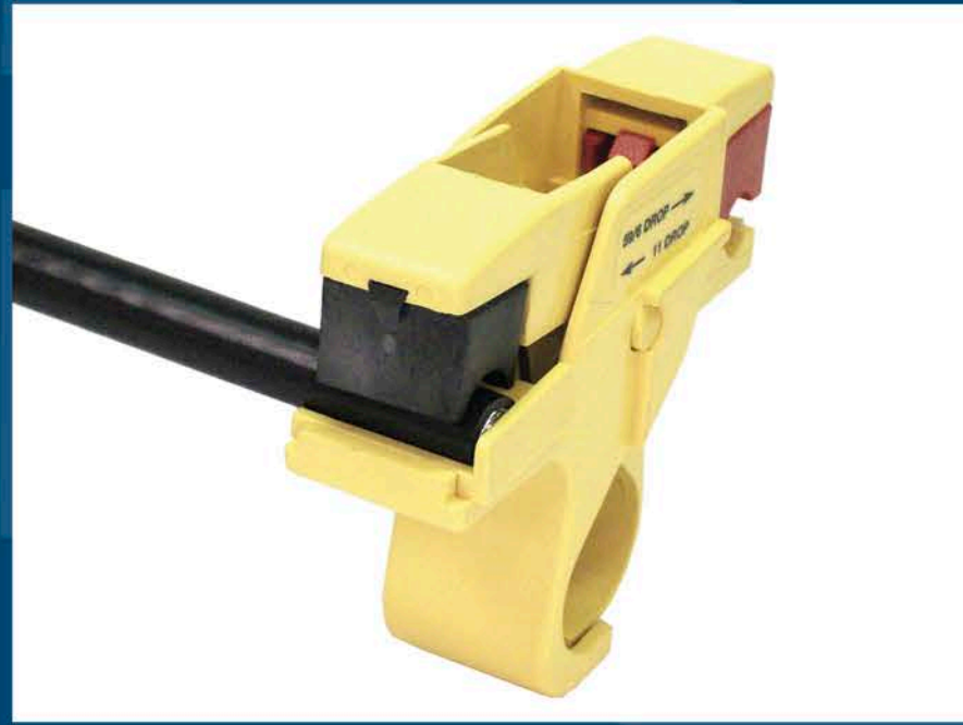
Using a fixed blade prep tool in good condition, prepare cable to 1/4" x 1/4" dimensions
