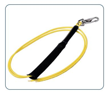
The SSF-PULLEYED is intended for use with simplex or duplex cables. The kit can also be utilized with Active Optical Cables (HDMI, DisplayPort, or USB), provided the connector head fits within the mesh sleeving. This kit also incorporates PVC-jacketed aramid yarns as the strength member. The pulling eye's clip rotates, helping to decrease twisting.
