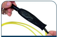
1. Flex cable sock mesh to an provide opening. Insert connector head. Ensure connector is toward the top of the mesh.
