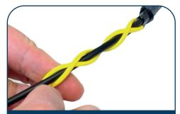
3. Braid the yellow strength members down the cable. Alternate crossing the two legs of the tubing above and below the cable.
