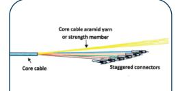
When possible, stagger connector terminations to reduce the pull sock diameter.
