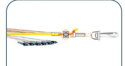
3. Insert aramid yarns into pulling eyelet and tighten screw. Ensure aramid yarns are parallel to the pulling eye and have no slack.
