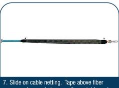
. Slide on cable netting. Tape above fiber connectors and at connection point to main cable jacket. Cable netting should not overly compress connectors.
