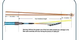
Cut core cable aramid yarns (yarns closest to fibers) so they extend 6" past the cable end or connectors.
