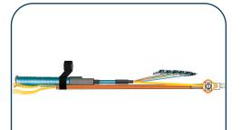
4. Tape pulling eye legs to cable. Using cable strippers, remove jackets from the pulling eye 1/2" from taped edge. Do not cut through the pulling eye's aramid yarns.
