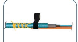
5. Braid the pulling eye's aramid yarns around the cable jacket 4-6 times at minimum. Knot ends and trim excess.
