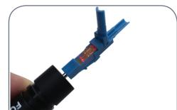
Place connector onto VFL. Ensure activator slide tab is in "open" position - slide towards rear of connector. Open hinge on connector.
