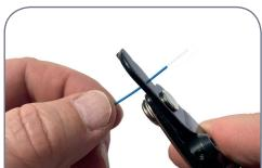
3. Using 125µm stripper opening and starting from fiber end, remove buffer and coating in 6mm increments to 30mm mark. Clean bare fiber with alcohol to a squeak.
