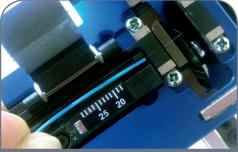
5. Cleave fiber measuring from  $900\mu m$  buffer coating. For SSF LC = 10mm.
