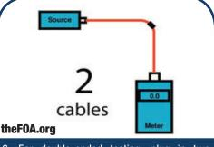
6. For double-ended testing, plug in two appropriate SC cables or two LC cables with adapters, one into OLS and one into OPM, with SC connectors or LC to SC adapters into OPM and OLS ports.<sup>1</sup>
