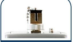
4. Plug REFERENCE cable into OLS. **Note: Do not look into laser while unit is on.**
