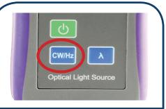
2. On the OLS press CW button until 1.0 KHz\* displays in lower right of the screen (see step 1A image).
