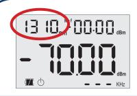
1B. Set OPM to same to same wavelength as the OLS unit. Press the wavelength button until desired value appears.
