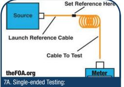
Unplug connector from power meter side ONLY. Place feedthrough SC or LC adapter, depending on cable being tested, on connector.
