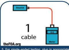
5. For single-ended testing, plug in appropriate SC cable or LC cable with SC to LC adapters (single mode or multimode according to the cable being tested) between OLS and OPM.
