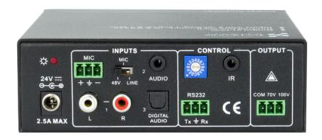
The TL-A70-40W is a compact-size amplifier that features alternative 70V or 100V output. It has 2 stereo inputs, 1 digital audio input and 1 MIC input. The TL-A70-40W can be controlled by button, IR, or RS232 command. It includes powerful functions, including ducking, EQ control, MIC mixer.
