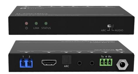
The TL-FO2-HDC2 is an HDMI 2.0 (18G signal) with HDCP 2.2 support fiber optic extender that can reach up to 300 meters (984 ft) over a duplex OM3 cable with common LC terminations. The unit supports HDMI video resolutions up to 4K@60, HDR video, IR or RS232 pass-through controls, multichannel audio, as well as ARC with optional optical audio embedding and/or de-embedding. The TL-FO2-HDC2 is also compatible with HDMI 1.3/1.4 content with HDCP 1.3/1.4 content protection.
