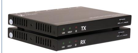
The TechLogix TL-TP100-HDC2 revolutionizes high-bandwidth HDMI signal distribution by leveraging HDBaseT technology to transmit 18G HDMI signals, including HDR and 4K@60 4:4:4, up to 100m (330 ft.) over standard twisted pair cabling.
