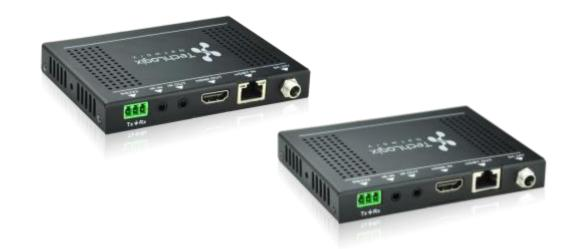
The TL-TP70-HDC is an ultra-thin extender set consisting of a transmitter (TL-TP70-HDC-T) and a receiver (TL-TP70-HDC-R). Using HDBaseT technology, the set transmits an HDMI signal to the receiver up to 70m distance via a Cat5e/Cat6A cable. Featuring bi-directional IR and RS232, you can control your display or source using included accessories. With bi-directional PoE power, you only need to connect the power supply on one end.
