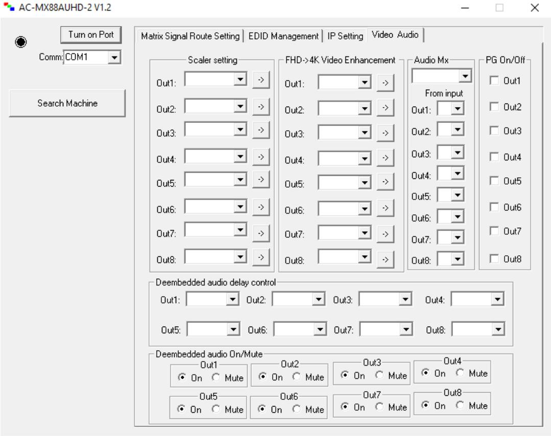
**Audio Mx** -- Set audio binding (FROM INPUT, FROM OUTPUT, MATRIX) and chose audio route when in MATRIX Mode.
