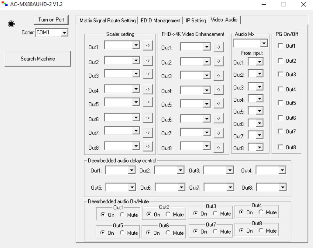
**Scaler Setting** -- This setting scales the HDMI output. You can also scale each output independently.
