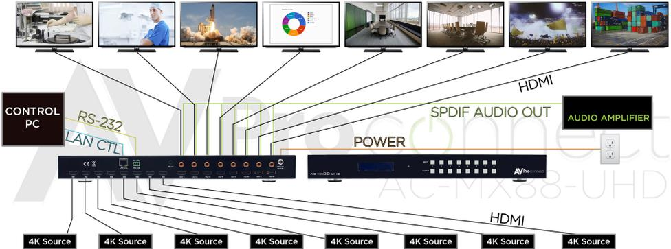
The AC-MX88-UHD is a 8x8 true HDMI matrix switcher, supporting HDMI2.0, HDCP2.2 and up to 4K video resolution and 10.2 GBPS bandwidth. It allows any source (BluRay player, UHD BluRay, satellite receiver, game station, etc.) to be shown on the any of the displays simultaneously.
