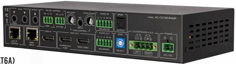
This multi-purpose device serves several functions in today's classroom, conference room, and boardroom. It includes an IP controllable 2 channel 25W Amplifier with microphone, line, HDMI and HDBaseT inputs, and full 18Gbps throughput (100M HDBaseT 10.2 Gbps). Outputs are scalable from 2K to 4K and 4K to 2K, and there are additional audio outputs for recorders, additional amplifiers, audio matrices, or other devices.
