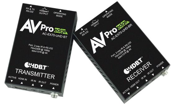
Anything but basic, this AVPro Edge extender is a cost-effective, state of the art, and reliable single CAT 70 meter extender featuring bi-directional power plus RS-232 and IR control. Pass 1080p HDMI signals 70 meters and 4K HDMI signal 40 meters all over readily available CAT-6a cable using HDBaseT technology.
