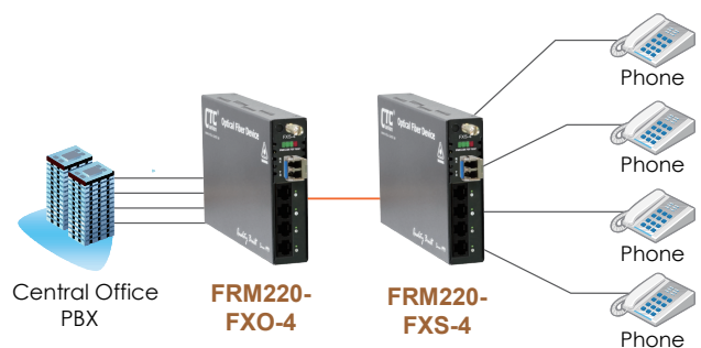
Voice transmission from 2km to 120km over fiber
