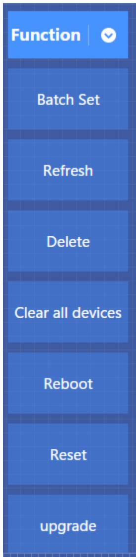
Batch Set: mean can configure the wireless AP's data in batch.
