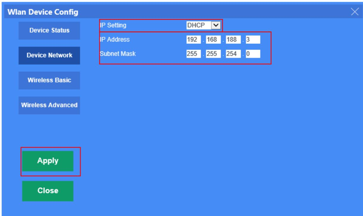
The screenshot shows the 'Wlan Device Config' dialog box with the 'Device Network' tab selected. The 'IP Setting' dropdown is set to 'DHCP'. The 'IP Address' field is set to 192.168.188.3 and the 'Subnet Mask' field is set to 255.255.254.0. Both the IP address and subnet mask fields are highlighted with a red box. At the bottom, the 'Apply' and 'Close' buttons are also highlighted with red boxes.
