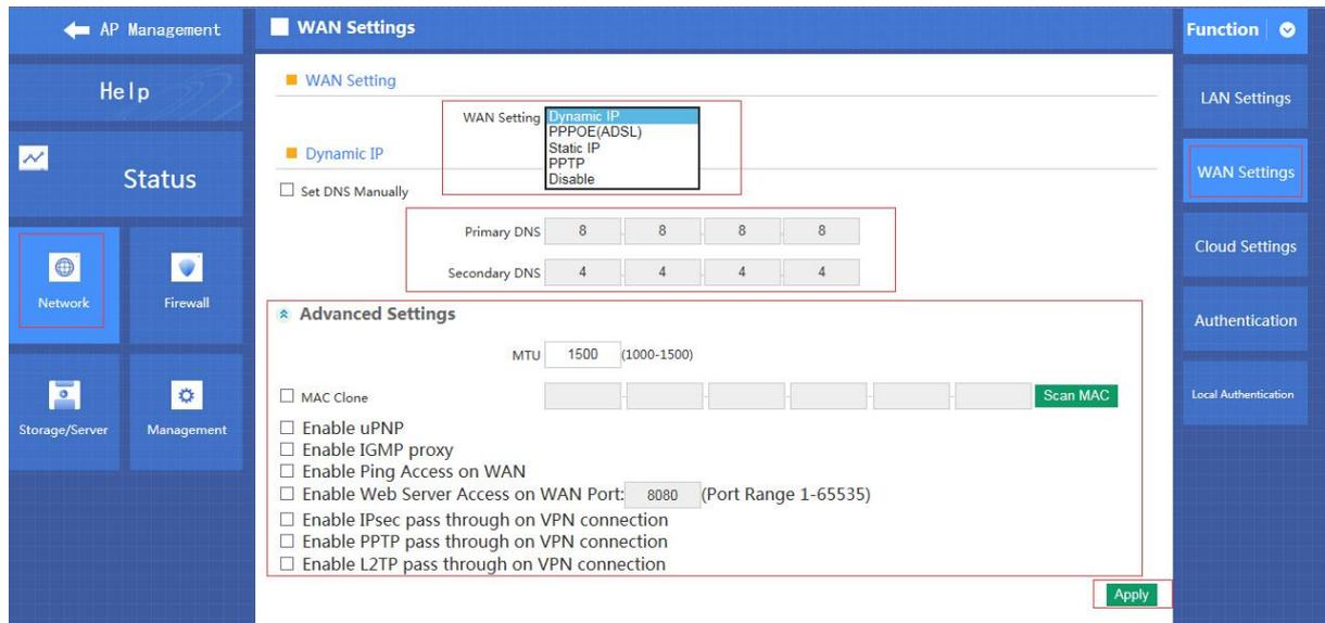
When select to intelligent gateway, NWAC7000 will have a router function, can work as a main router with Gigabit WAN/LAN port. It support Dynamic IP, Static IP; PPPOE; PPTP.
